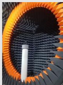
Anechoic Chamber 400 MHz - 18 GHz
