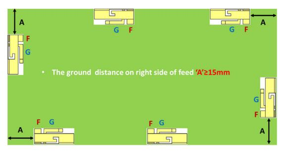
Figure 8: optimal antennas placement for 1000146 on a large PCB
