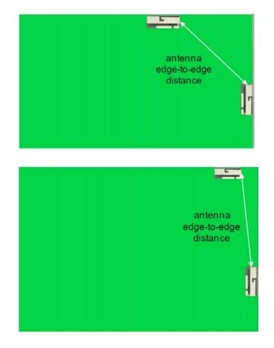
Figure 16: Recommended Layout for MIMO Applications
