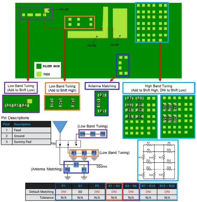
Figure 4: 1000146 Antenna Matching Structure (Major Tuning Structure)
