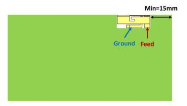
Figure 7: optimal single antenna placement for 1000146
