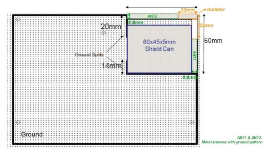
Figure 19: A Typical MIMO Configuration Example
