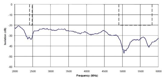
Figure 20: Measured Isolation Between Two 1000146 MIMO Antennas
