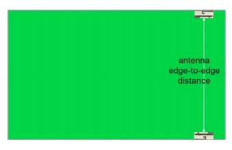
Figure 18 : Recommended guidelines for two antennas placed on opposite edges of PCB
