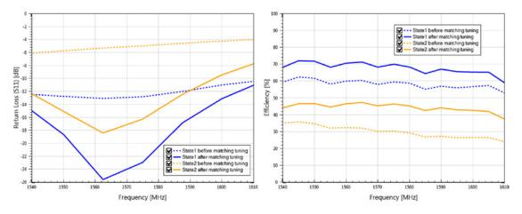
Figure 7: Matching Tuning adjustment for 1001011
