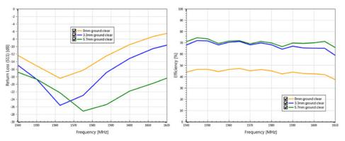
Figure 8: Ground clearance changes for 1001011
