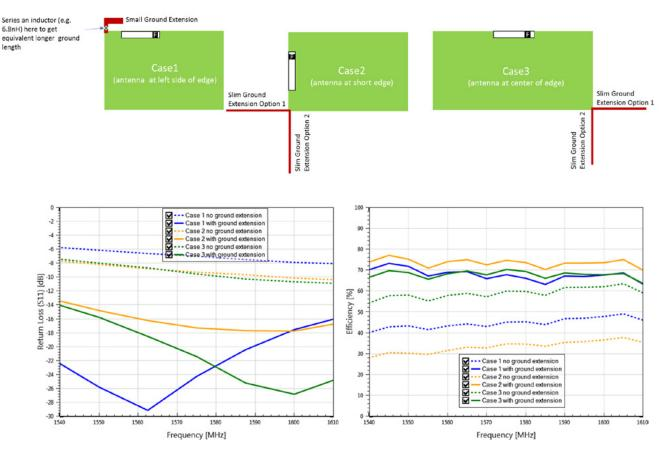
Figure 10: 1001011 antenna performance improvements with ground extensions
