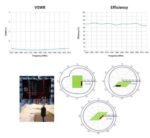
Figure 4: Typical Performance for 1001011\_Off-Ground
