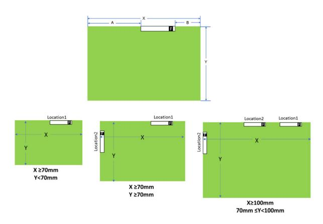
Figure 6: Optimal placement of the 1001011 on a PCB
