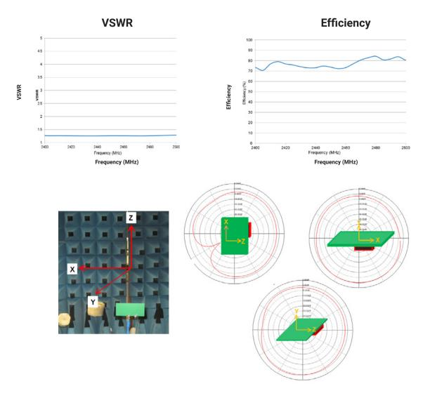
Figure 4: Typical Performance for 1001013-02 (Off-Ground)
