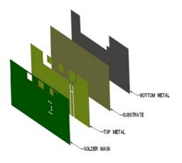
\* VIAS: Diam. 0.2mm, (no vias on transmission lines). Via holes must be covered by solder mask
