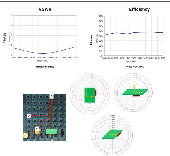
Figure 5: Typical Performance for 1001013-1 (On-Ground)
