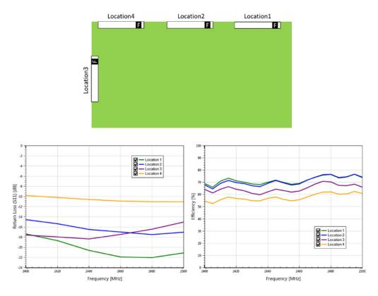
Figure 9: 1001013 antenna on different board locations
