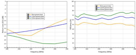
Figure 8: Ground clearance changes for 1001013
