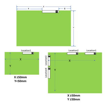
Figure 6: Optimal placement of the 1001013 on a PCB
