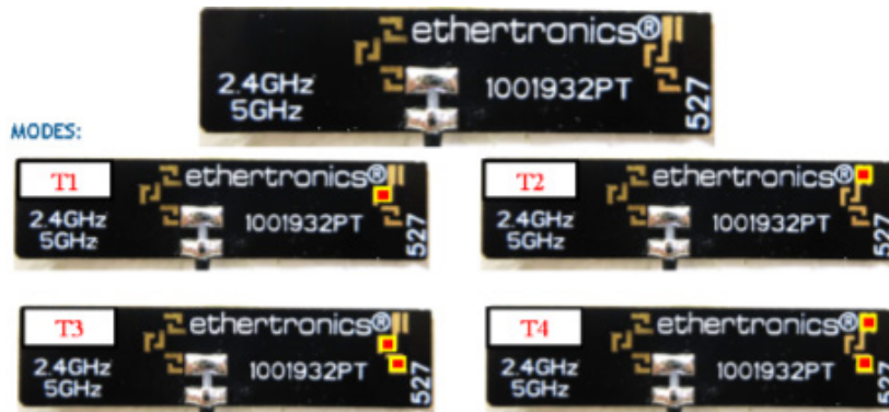
Connection: Bridge with solder to tune antenna
