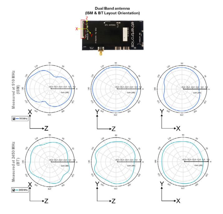
Figure 6 : 1002427 Antenna Typical Performance for ISM & BT Dual Band
