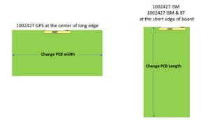
Figure 15 : PCB Width or Length Change
