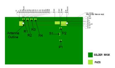
\* VIAS: Diam. 0.2mm, (no vias on transmission lines). Via holes must be covered by solder mask
