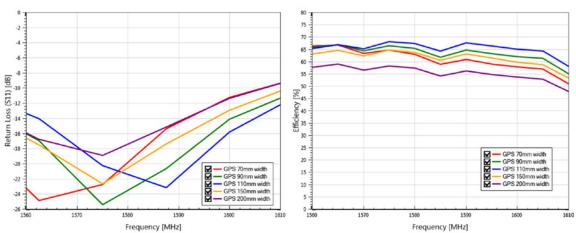
Figure 16 : 1002427 GPS ONLY performance varies with different PCB width
