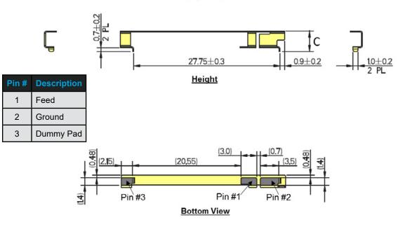
Figure 1 Antenna Dimensions for the 1002427
