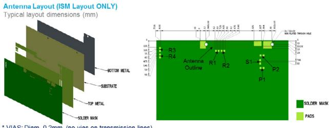
\* VIAS: Diam. 0.2mm, (no vias on transmission lines). Via holes must be covered by solder mask Pin Descriptions
