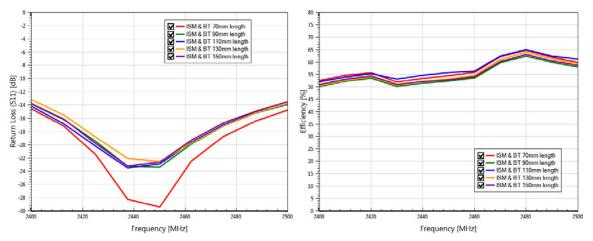
Figure 18 : 1002427 ISM & BT performance varies with different PCB length
