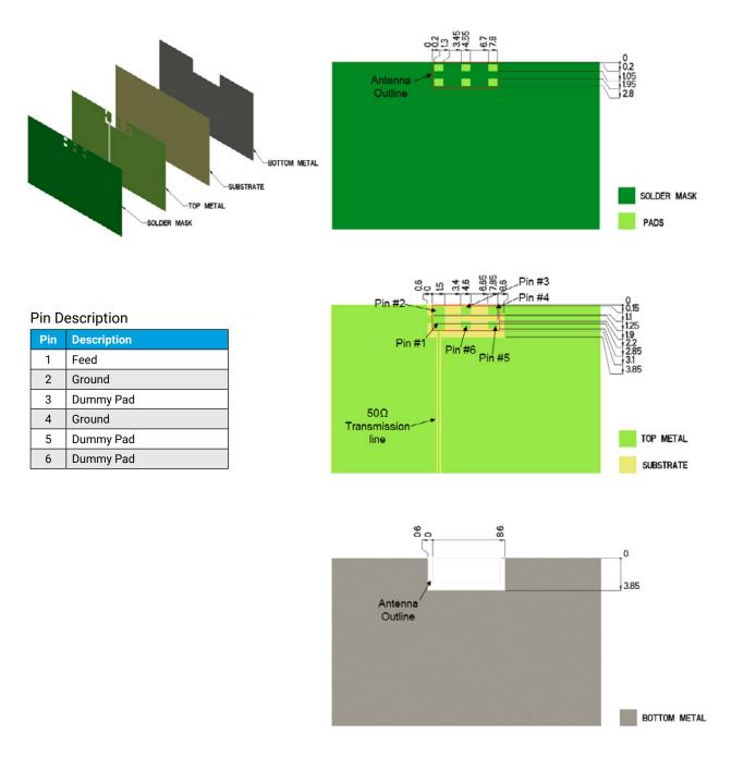
KYOCERA AVX provides antenna layout files in .DXF format. This is a universal file format and should be converted into your specific file format.
