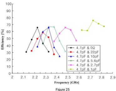
A low value Inductor can be used to shift the frequency lower;
