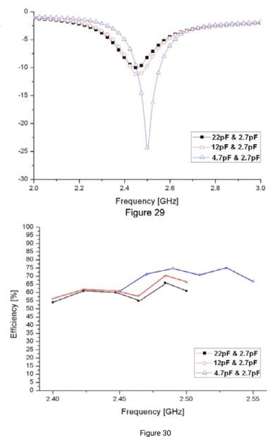
See Figure 29 to the right and Figure 30 below to see the results of changing the Capacitor value on Return Loss and the corresponding Efficiency.
