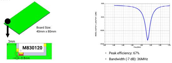
Recommended board layout change in red circle: needs to fill the gap by 0.5mm to optimize the performance.
