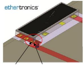
Shorting pin and feed pin are shared inKYOCERA AVX ceramic antenna
