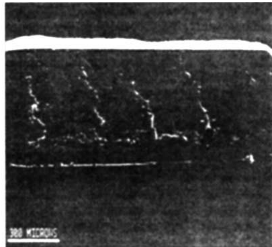
Figure 17. Micrograph of Acceptable Failure Mode with Fracture Mode Running Over Several Pt Plates
