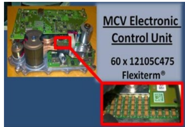
Figure 7: Example MLCC Application in Automotive ECU
