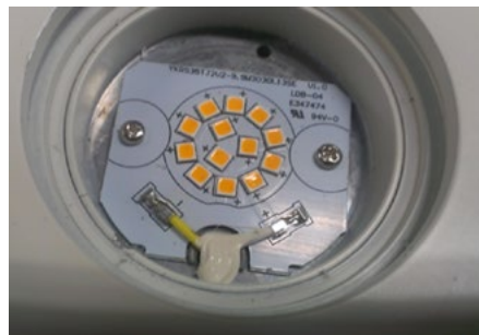
Figure 3: Example of a one-piece connector replacing hand soldering
