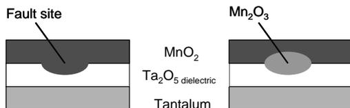
Fig.3. The fault site in dielectric after MnO<sub>2</sub> self-healing process
