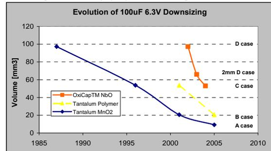
Fig. 1. Time evolution of 100 $\mu\text{F}$  6.3V downsizing
