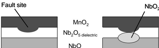
Fig.5. The NbO<sub>2</sub> self-arresting process
