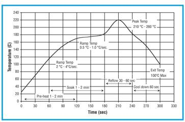
Figure 1. Typical Infrared or Convection Reflow Profile
