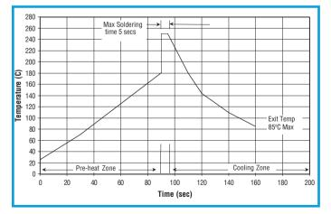
Figure 2. Typical Wave Solder Profile
