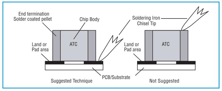
Figure 4. Recommended soldering techniques
