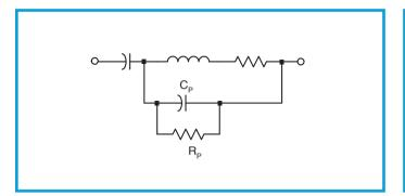
Figure 2. Equivalent Circuit Model
