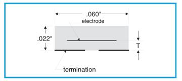
Figure 2. Typical longitudinal cross section.
