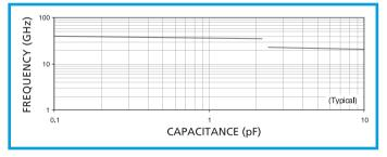
Figure 1. Typical first parallel resonant frequency.
