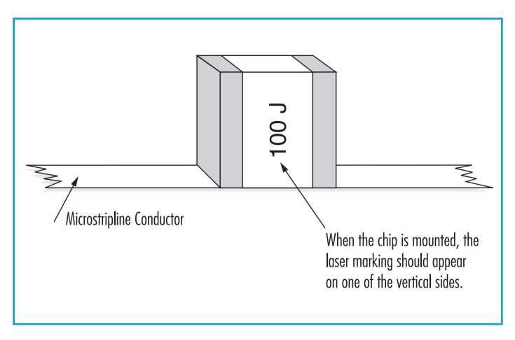
You may order a HN or HS style capacitor having narrow microstrip leads such that the capacitor plates are in the orientation shown in the illustration.
