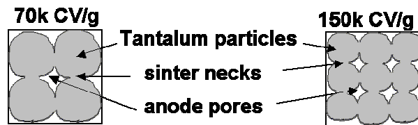
Fig 3 : Schematic model of anodes from two different CV/g powders showing significantly finer structure (sinter necks, pores, grains) for higher CV/g powder.
