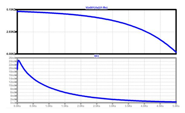
Figure 6: Side by Side view of supercapacitor's current and NTC resistance in a 10F supercapacitor and  $R_{150@25C}$  NTC system
