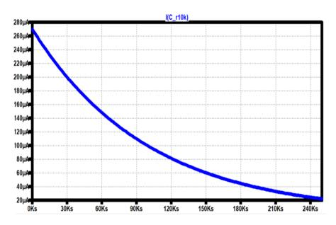
Figure 2: Spice simulation of 10F supercapacitor with a  $10K\Omega$  series resistor
