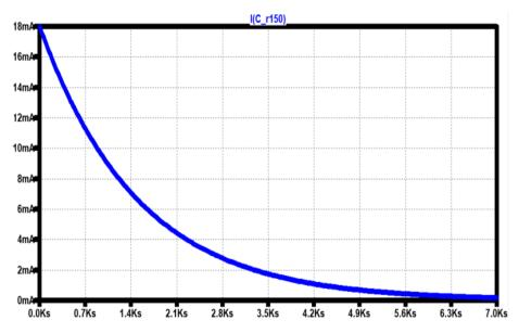
Figure 3: Spice simulation of 10F supercapacitor with a  $150\Omega$  series resistor
