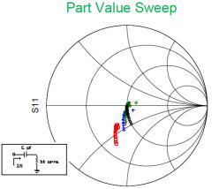
Legend: 14mil FR4, + 31mil FR4,  $\diamond$  59mil FR4, O Ideal Model S11 at 2 GHz for capacitor values from 3.3 to 1000 pF on various substrates compared to an ideal capacitor response.
