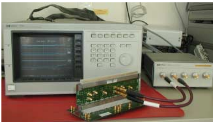
Fig. 16 TDR measurement setup
